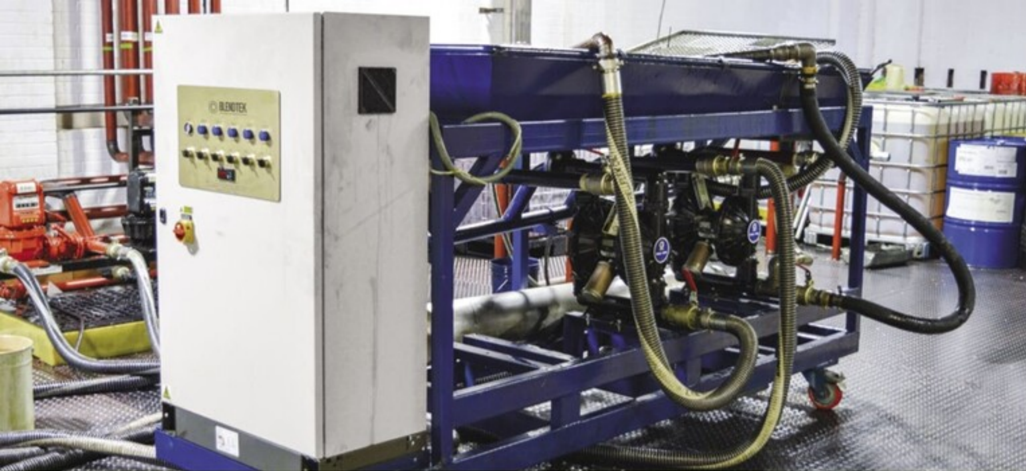
Ultrasonic controller and cavity on a trolley at Witham Group's blending plant. Photo courtesy of Witham Group
