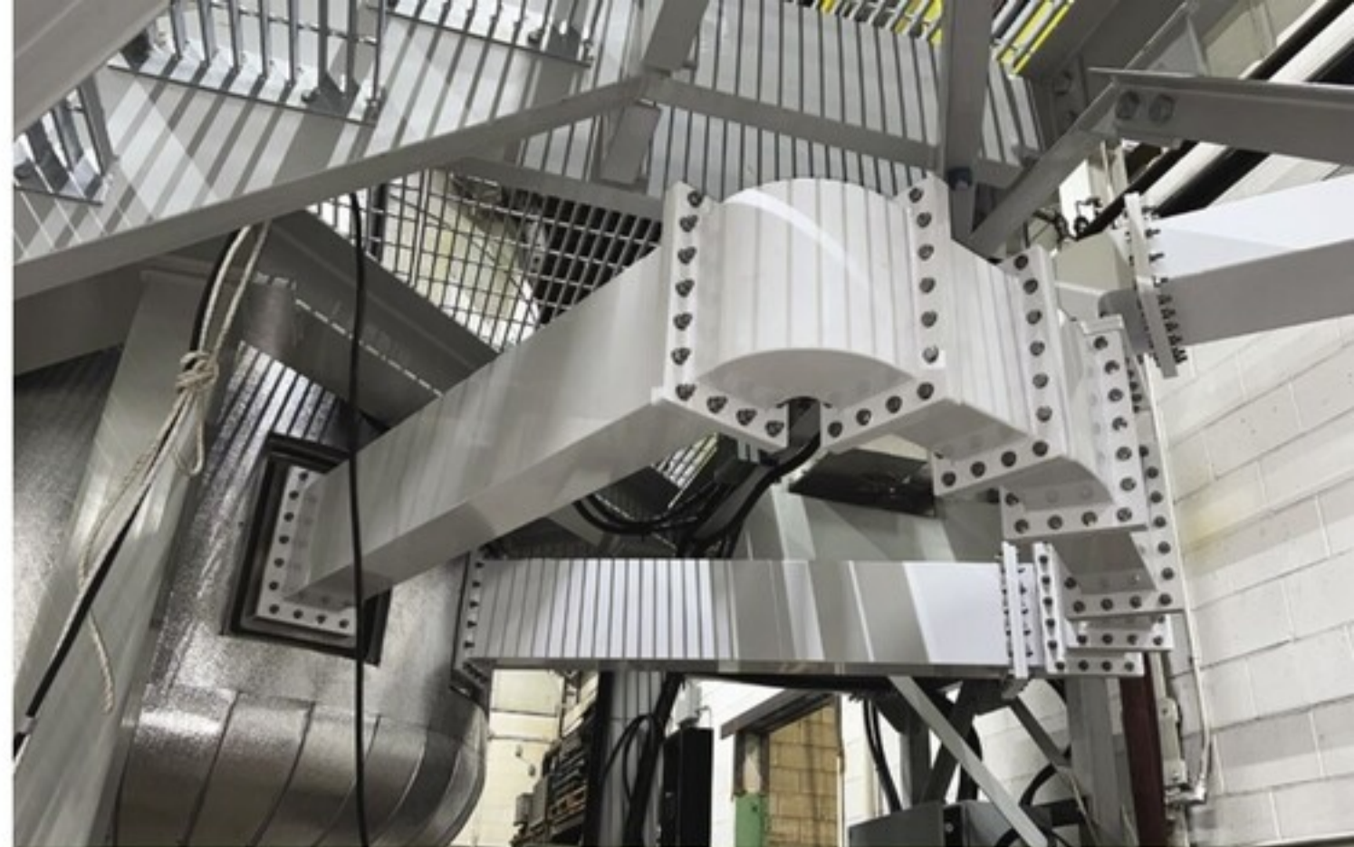
Rear view of the Patterson microwave kettle showing the attachment of the waveguides near the base. Photo courtesy of Patterson Industries (Canada)
