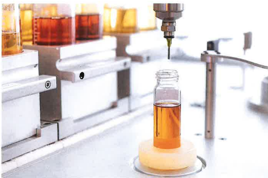
Figure 5. High-throughput lubricant blending robot. Figure courtesy of Novvi, LLC.
