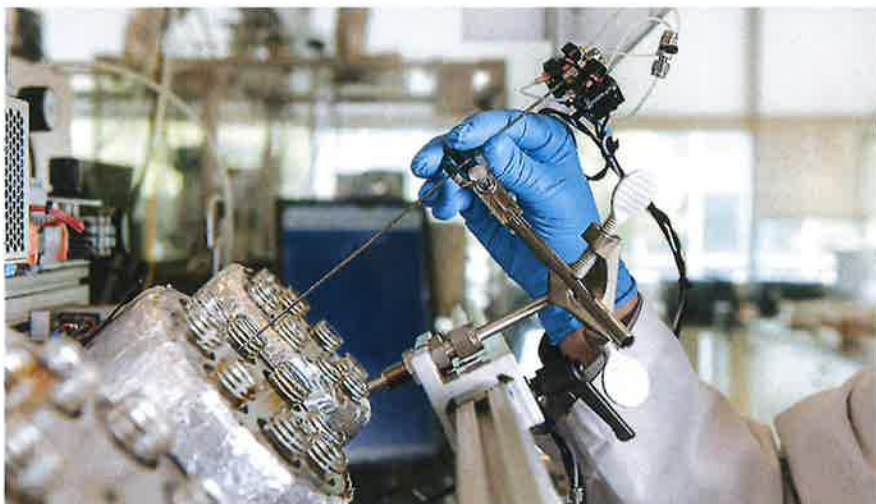
Figure 2. Multi-channel accelerated aging test for bulk and thin film oxidation. Figure courtesy of Novvi, LLC.
