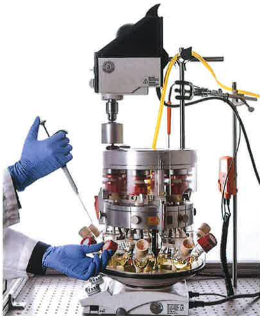
Figure 1. Multi-channel accelerated oxidation test. Figure courtesy of Novvi, LLC.
