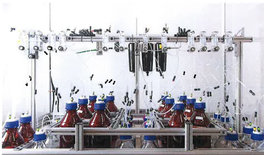
Figure 3. Multi-channel OECD 301b biodegradation testing system. Figure courtesy of Novvi, LLC.
