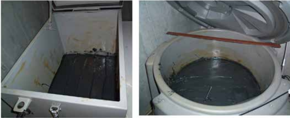
Figure 3: The lubricators from the two OEMs were filled with the same quantity of grease and tested at the same temperature in the environmental chamber.
