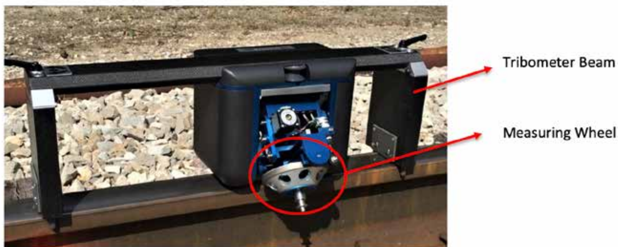
Figure 8: A close-up view of the tribometer's measuring wheel at the measuring position
