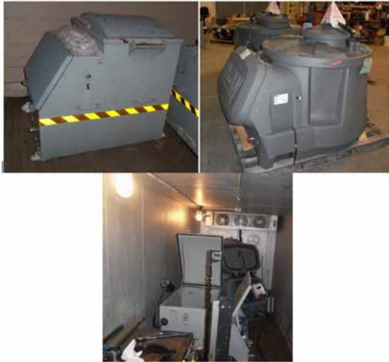
Figure 2: The high-pressure Unit 1 (top right) and the low-pressure Unit 2 (top left) were tested in the environmental chamber (bottom).
