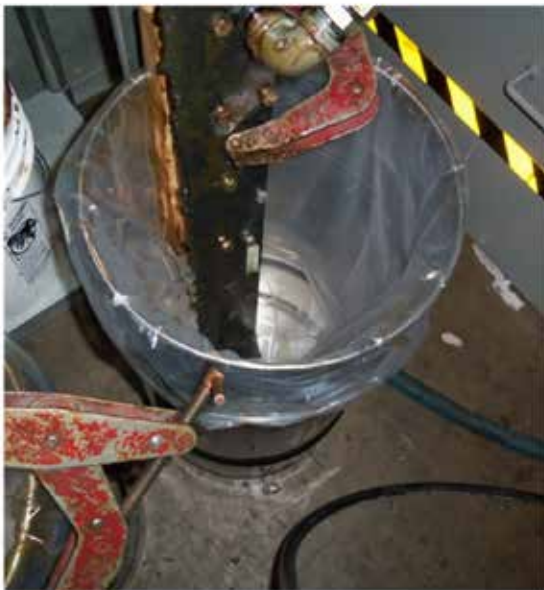
Figure 3: The lubricators from the two OEMs were filled with the same quantity of grease and tested at the same temperature in the environmental chamber.
