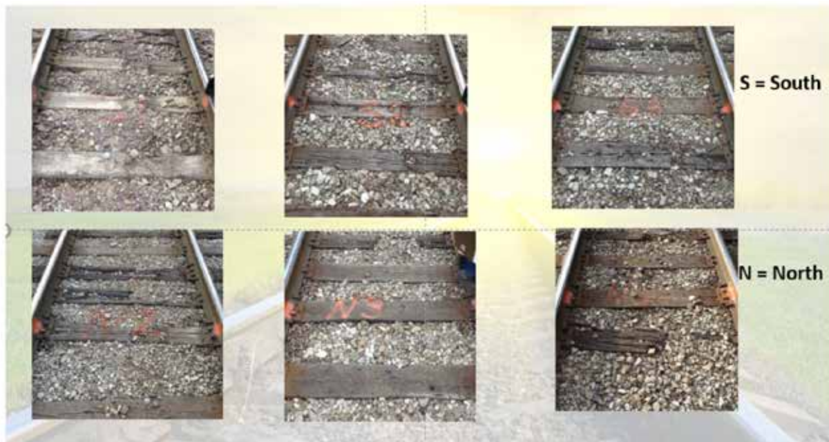
Figure 9: Example of mark ings on the track locations where friction was measured
